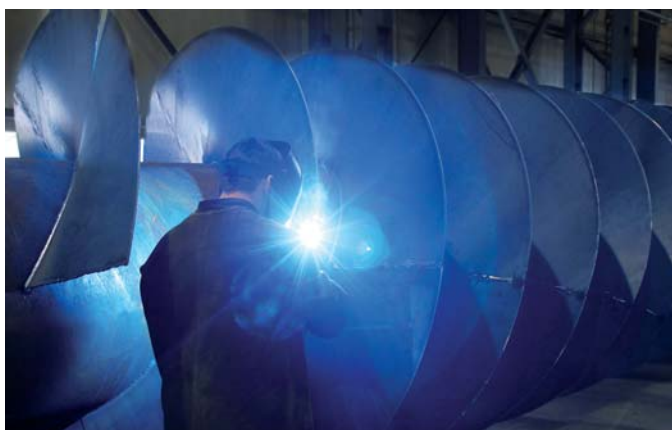
. . . then welded onto the body of the screw, and . . .
