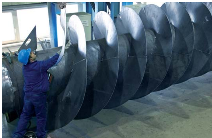
The blades of the screw pumps are curved and aligned precisely. . .
